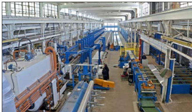
Figure 1. Overview of the first 25 MN, 9 inch press line installed at the Livonia facility.
