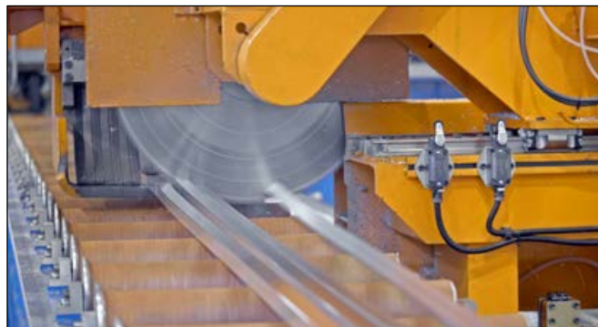
Figure 2. The automated flying hot saw cuts the profiles as they exit the press.
